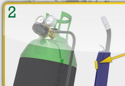
Press trigger to release pressure in the hose.
